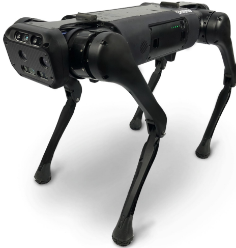
Figure 1.1: Aliengo robot model from Unitree [12]. Each leg has a hip (joint closest to the base), thigh, and calf (closest to the foot) motor angle that can be controlled. For the remainder of the thesis the order in which joints are considered is: front right, front left, rear right and rear left leg.
